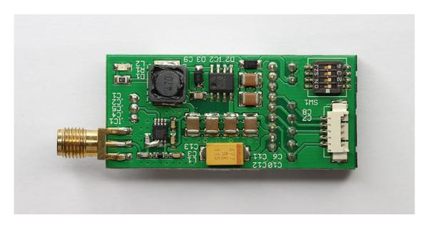
Fig 2. Bottom side of ImmersionRC 600mW 5.8GHz audio/video transmitter.
