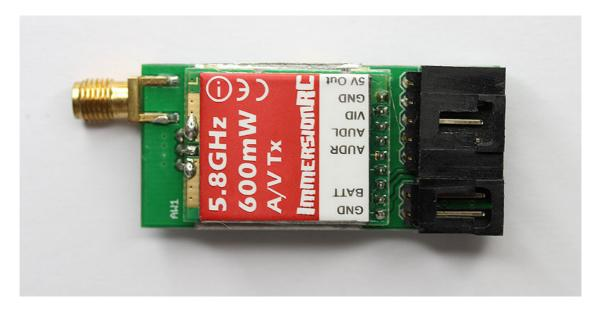
Fig 1. Top side of ImmersionRC 600mW 5.8GHz audio/video transmitter.
